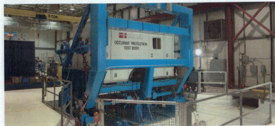
The Horton body was subjected to 14 rollover impacts while establishing a baseline, and then testing HOPS. The body retained its structural integrity through it all.
