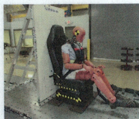
Like any collision protection system, HOPS is effective only when occupants are wearing seat belts. CPR, head and aft bench seat belts have detachable four point belts to enhance mobility.
