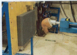
A head-strike cannon is used to test the HOPS cushion system
